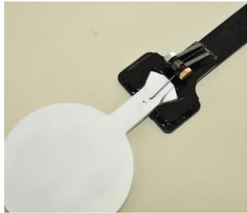
5) Install each target by sliding the point on the target sideways under the spring. Insure that you do not jostle the installed targets causing them to drop out. The targets are heavy and could cause injury if they hit you.
