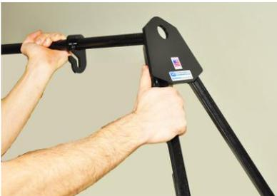
4) Insert legs into other side plate and lay it on the ground near the end of the bar. Lift end of the bar and slide the second leg/side plate assembly onto the bar. Adjust legs/side plates until the entire frame is stable.
