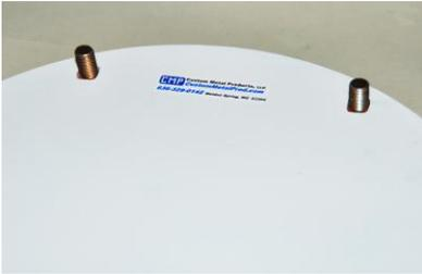
1) Lay target face down on a table, insert the Grade 8 carriage bolts with the round head on the face that is exposed to bullet strikes. The two grade 8 carriage bolts, washers and locknuts are shipped with the Gong stand. Do not use any lower grade bolt, as they will be damaged by bullet strikes.
