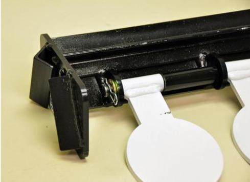
2) If it ever becomes necessary to remove or replace a target, remove the hitch pin and washer from each end and slide the 1/2" diameter shaft out through the targets, spacers and mounting brackets.
