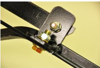
3) Install both folding legs with the split lock washer and locknut on the inside of the legs. Tighten so the legs move, and the lock washer provides enough friction to hold them in place.
