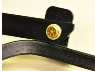
2) Install leg with radiused side toward the post, using the 1/2-13 hex head grade 8 bolt and hardened washer on the outside of the leg.
