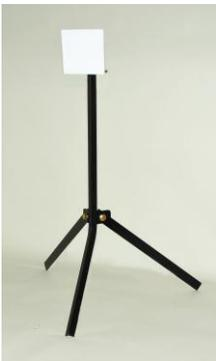
6) Stand target in desired location, adjusting the folding legs to accommodate uneven ground and to make post vertical. The legs may be locked in place by fully tightening the locknuts. The stand and target is now ready for use.
