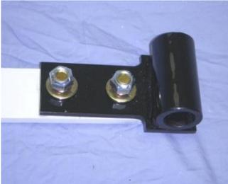
2) Set the target mounting bracket down onto the bolts, and install hardened flat washers and locknuts, firmly tighten the locknuts
