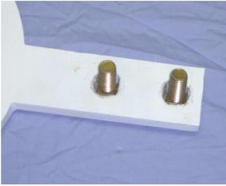
1) Lay target face down on a table, insert the Grade 8 carriage bolts with the round head on the face that is exposed to bullet strikes. The two grade 8 carriage bolts, washers and locknuts are shipped with the Swinger frame. Do not use any lower grade bolt, as they will be damaged by bullet strikes.
