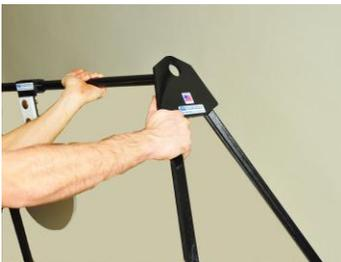
5) Place other leg/side plate assembly on the bar. Adjust side plates / legs until the entire swinger assembly is stable. Read the Target Care and Use instructions on the back side of this sheet. The target is now ready for use.
