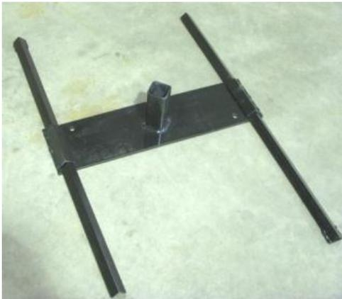
3) Place the static base on the ground and slide the stabilizer legs into the pockets.
