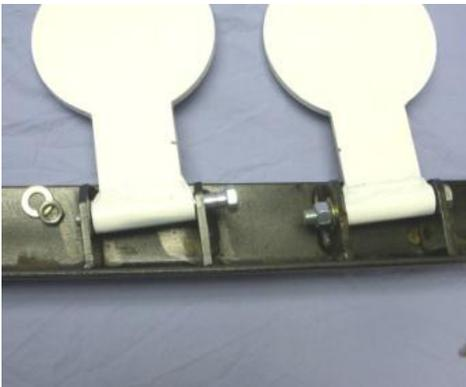
2) Place target with tube between the holes in the mounting brackets, slide a bolt upwards through the bracket, tube, then other bracket, and place the washer and locknut on top of the bolt. Tighten the locknut firmly, ensuring the target moves freely all the way from one side to the other. Repeat for all targets
