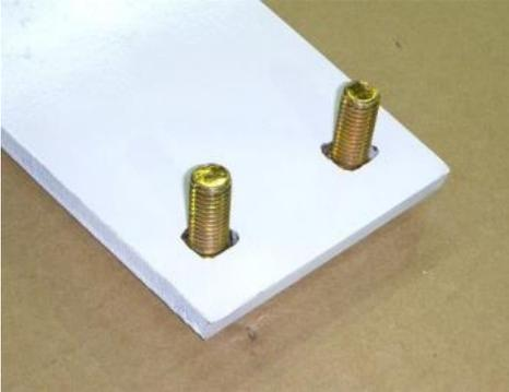
1) Lay target face down on a table, insert the Grade 8 carriage bolts with the round head on the face that is exposed to bullet strikes. The two grade 8 carriage bolts, washers and locknuts are shipped with the Auto Reset Base. Do not use any lower grade bolt, as they will be damaged by bullet strikes.
