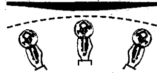
WRONG WAY - Stiff wrist makes an arc, building up paint in center.
