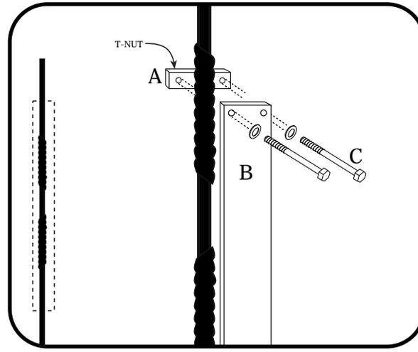
Insert bolt with washer (C) through mounting board (B) and screw into T-nut on opposite clamp (A). The clamp with the T-nut should be on the outside of the post. Repeat at the other end of the clamp. Mount gate according to instructions.
