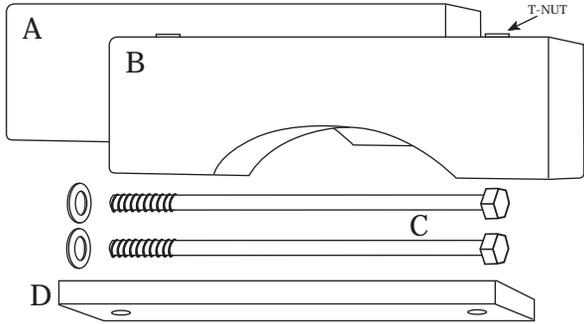
Wood Clamps provide a means for attaching your gate to a post without damaging the post with screws. Please follow these procedures to install a CARDINAL GATE.
