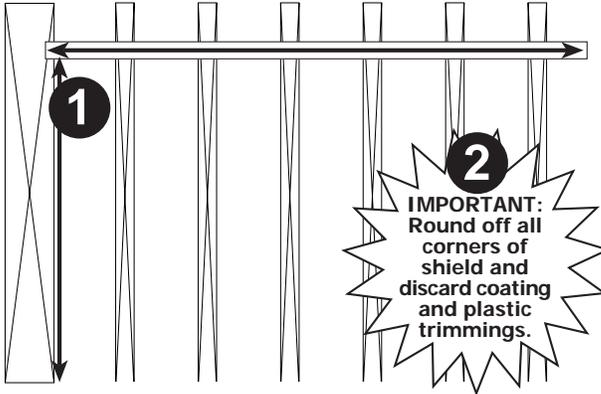
1. Measure the length and the height of the section of the banister to be covered. Make sure the plastic reaches all the way to the floor and the top of the railing. Add at least 2 inches for overlapping at both ends for newels and add 6 inches if one side is a wall (Refer to diagram on **STEP 5**).
