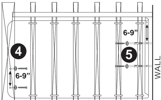
4. Deck Shield™ may be fastened to the endpost with cable ties. For a more secure attachment to the end post, drill a 1/16 inch hole through the plastic and into the endpost, then secure the plastic with the screws and washers provided (**C**). Space screws or ties no more than 6 to 9 inches apart.
