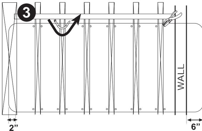
3. Hold plastic in place with ends overlapping endposts (2 inches) and/or wall (6 inches). Make marks on the plastic on either side of one of the baluster posts no less than 1/2 inch from the top edge. Use hole punch (**B**) to punch holes at your marks. Press hard, you may need to use both hands. Use cable ties (**A**) and insert through the holes from the backside of the plastic. Tighten the tie, and cut off the excess cable tie. Repeat this process on top and bottom of each baluster.
