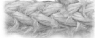
Rope must be replaced
