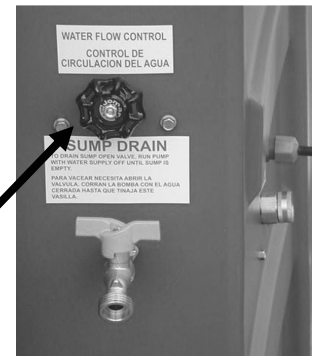
Open water flow valve 1 1/4 turns to allow water to fill reservoir.
