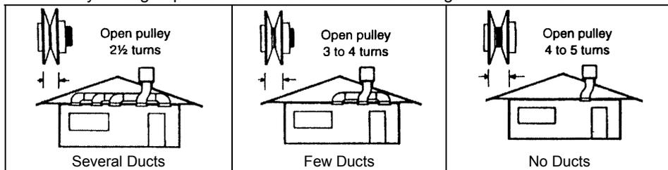
Set Pulley for Air Flow Resistance
