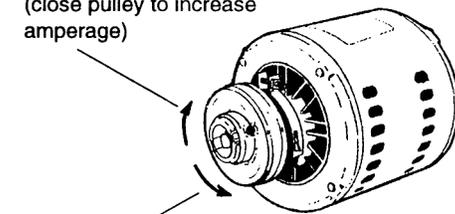
Smaller Diameter Pulley
