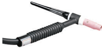
Weldcraft® Legacy™ 17 Replacement TIG Torch 1712RESYLGC #245271 12.5 ft. (3.8 m) TIG torch with backcap, ceramic gas cup, 3/32 in. (2.4 mm), collet and collet body, and 2% ceriated tungsten.
