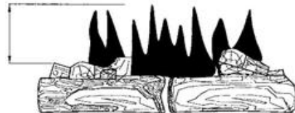
Figure 18 - Incorrect Flame Pattern with Control Knob Set to High Flame (5)
