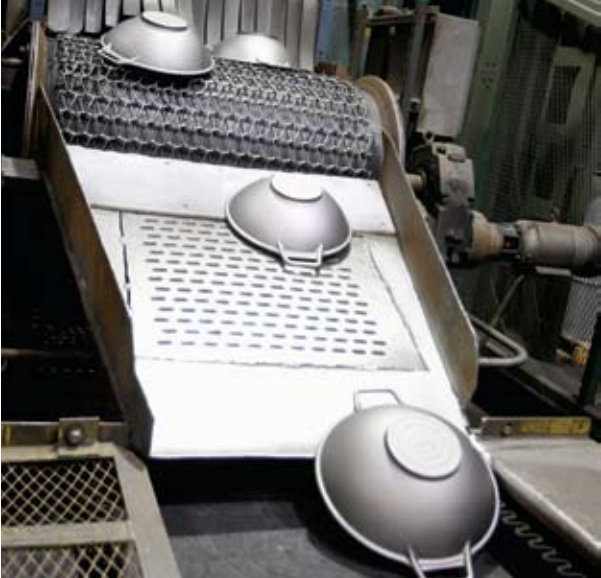
Cast-iron woks ride the conveyor en route to their third and final cleaning. The seasoning process turns cast iron black.
